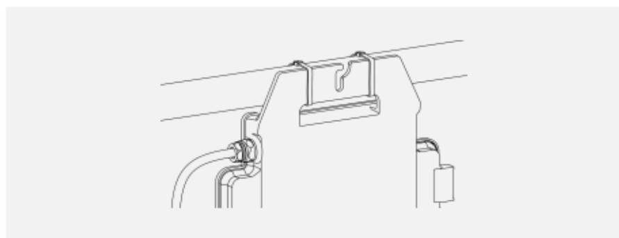
The Microinverter EZ1 can be installed on the balcony wall or fixed to the railing using cable ties. Select an appropriate installation method based on your actual scenario to ensure that the EZ1 is securely installed.
