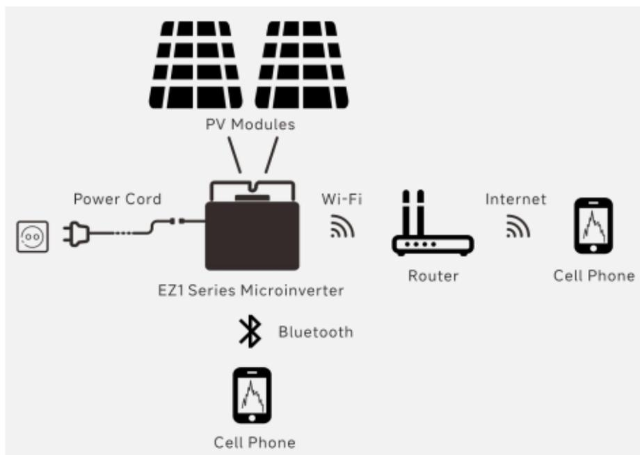
The EZ1 series APsystems Microinverter is used in balcony and DIY systems which comprised of the below key elements:
