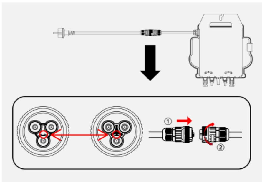
Insert the microinverter AC connector into the power cord connector.
