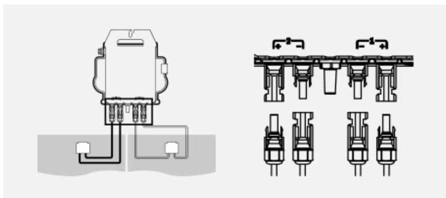
When plugging in the DC cables, the microinverter should immediately blink green ten times. This will happen as soon as the DC cables are plugged in and will show that the microinverter is functioning correctly. This entire check function will start and end within 10 seconds of plugging in the unit, so pay careful attention to these lights when connecting the DC cables.
