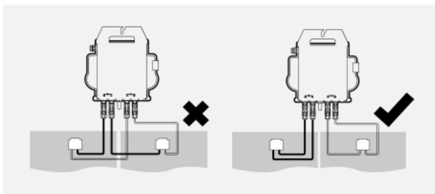
**NOTE:** Each PV panel must be carefully connected to the same channel. Make sure to not split positive and negative DC cables into two different input channels: microinverter will become damaged and warranty will not apply.
